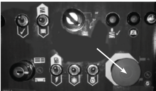
Figure 9.2 - Ground Control Box Emergency Stop Switch
