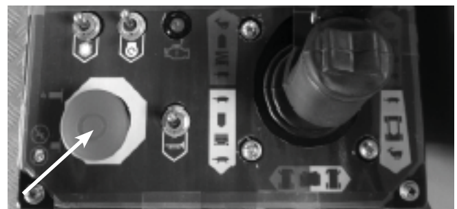
Figure 8.2 - Emergency Stop switch at Platform Control Box
